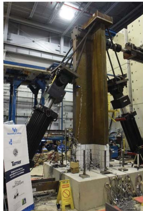
Fig. 5. Finished test setup of T-shaped wall specimen.
