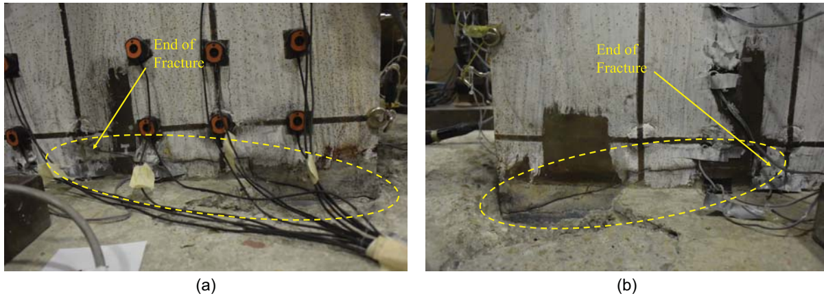
Fig. 10. Fractures after test is complete and local removal of concrete at (a) north face of the web (NW); and (b) south face of the web (SW).
